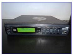
A sound module, which requires an external controller to trigger its sounds. These devices are highly portable, but their limited programming interface requires computer-based tools for comfortable access to their sound parameters.
