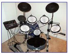
Drum controllers, such as the <u>Roland V-Drums</u>, are often built in the form of an actual drum kit. The unit's sound module is mounted to the left.
