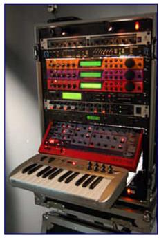
MIDI allows multiple instruments to be played from a single controller, which makes stage setups much more portable. This system fits into a single rack case, but prior to the advent of MIDI would have required four separate keyboard instruments, plus outboard mixing and effects.
