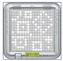
Yamaha's <u>Tenori-on</u> controller allows arrangements to be built by "drawing" on its array of lighted buttons. The resulting arrangements can be played back using its internal sounds or external sound sources, or recorded in a computer-based sequencer.
